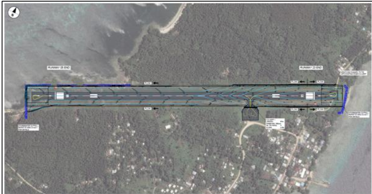
Figure 39: Drainage concept design showing much of the runway drainage discharge into the SW coastal environment
