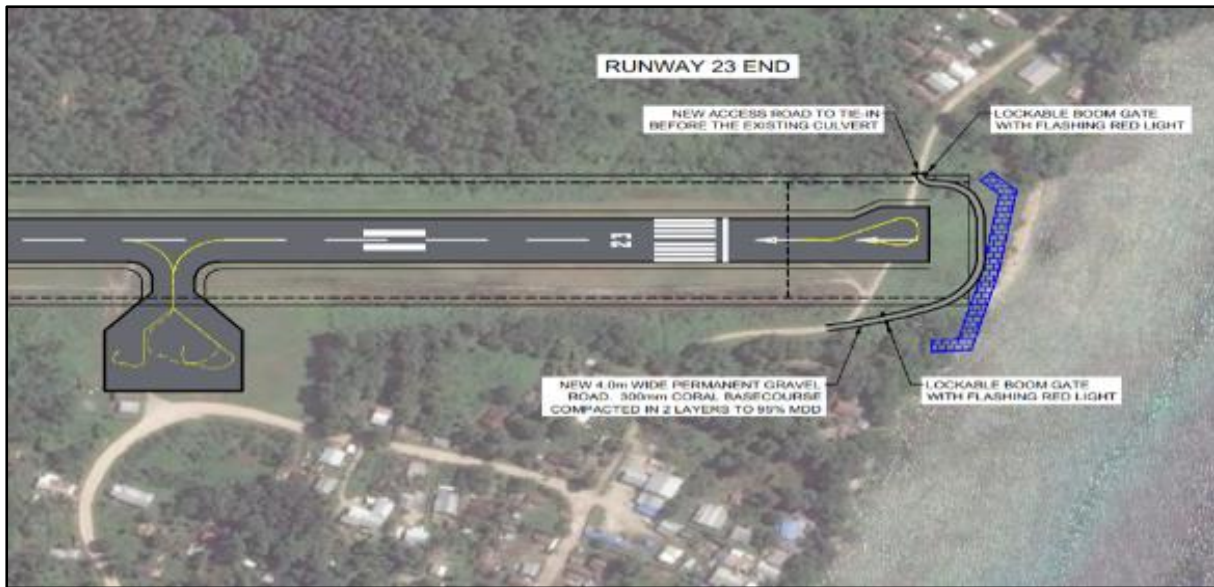
Figure 6: Public access road around the northern perimeter of the runway with a lockable boom gate
