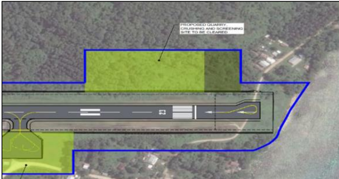
Figure 8: Proposed site for project quarry (yellow) within the airfield leased boundary (approx. boundary shown in blue)
