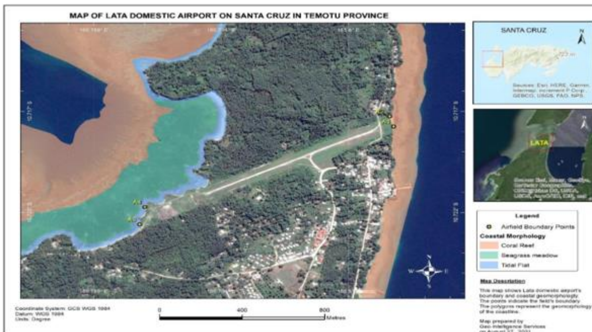
Figure 21: Map showing the coastal morphology and the habitat types along the Santa Cruz airport marine area. (Source: Marine Survey and Assessment Report for Santa Cruz Airport Upgrade Project)
