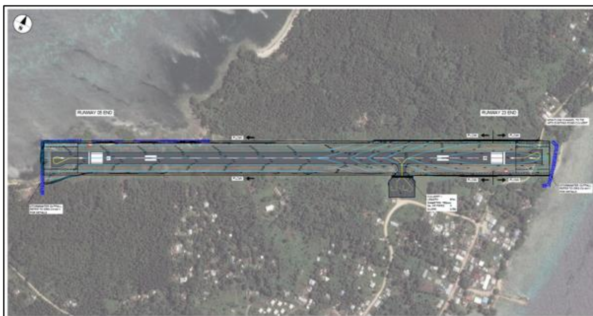
Figure 44: Drainage concept design showing much of the runway drainage discharge into the SW coastal environment
