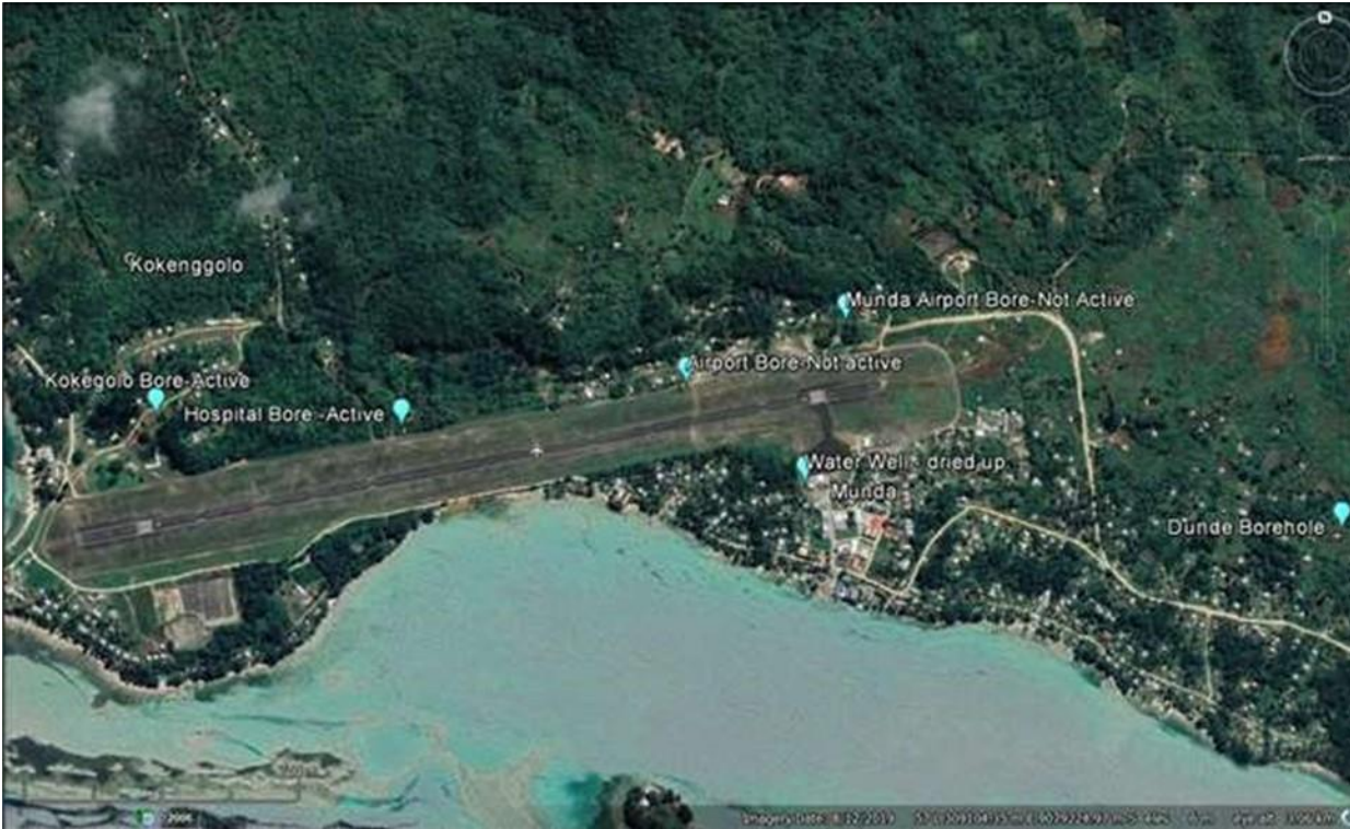
Figure 8: Water supply boreholes in Munda (source from Solomon Water)
